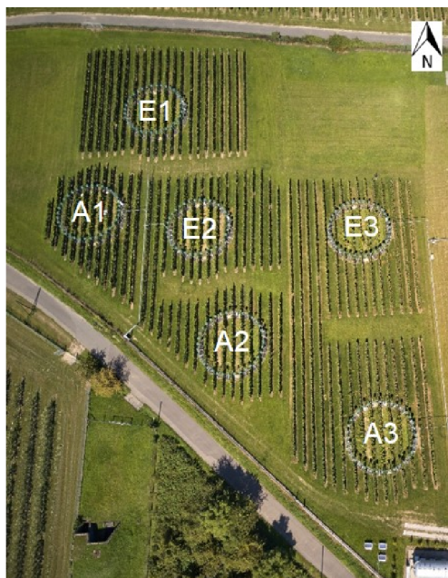
Supplementary Figure 2. VineyardFACE experimental site at Hochschule Geisenheim University with corresponding CO 2 tank (bottom right corner). The FACE-rings A1, A2 and A3 were related to ambient CO 2 level (aCO 2 ), whereas E1, E2 and E3 were related to elevated CO 2 level (eCO 2 ). Associated numbers to FACE-rings 1, 2 and 3 were defined as blocks.
