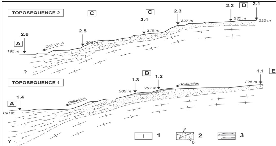
**Figure 5/** Characterization of the microterroirs (A to E) integrating topographic, pedo-geological and microscale climatic zoning data (not at scale). Symbols: 1, molassic basement; 2, altered molassic basement (a: clay dominant; b, sand dominant); 3, solifluction lobes.
