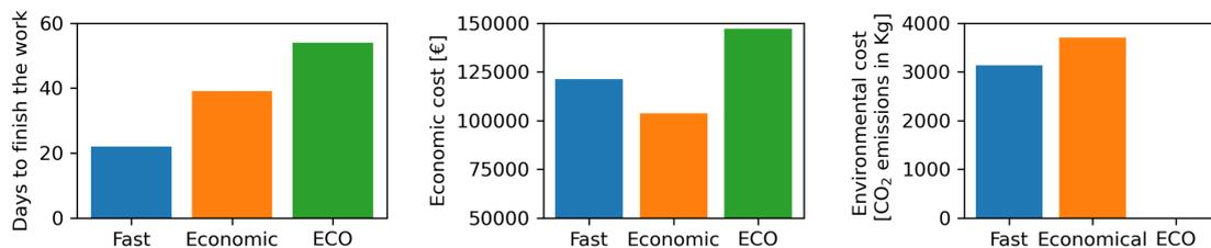
Figure 2: Costs associated with the three schedules generated by prioritizing time (blue), economic cost (orange) or environmental impact (green). Each figure represents a different total cost: time to finish all the works (left), total economic cost (middle), total environmental impact (right).
