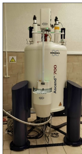
Figure 1. Magnet unit of the BRUKER NMR spectrometer Avance™ NEO 700 (Germany) at the RUDN University (Moscow).
