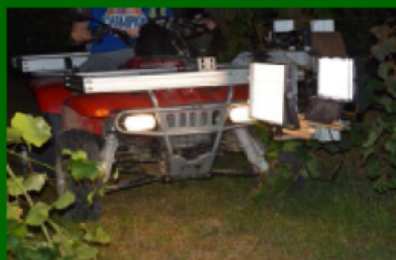
Figure 1. Mobile platform used for image acquisition on-the-go in the commercial Pinot noir and Macabeo vineyard moving at 5 km/h
