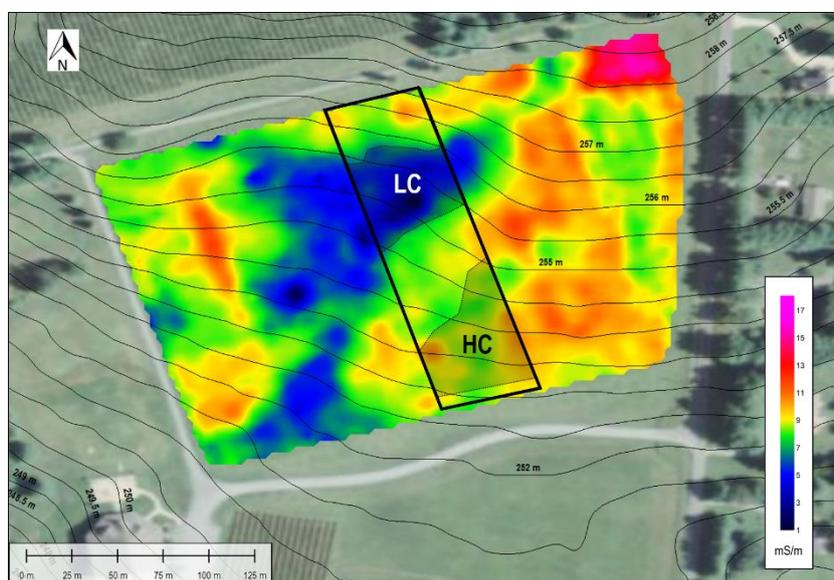
**Figure 2: Electromagnetic conductivity map showing soil variability in study area. The two harvest zones (labeled LC and HC) are distinguished in the field by differences in soil properties which correlate to soil EC.**
