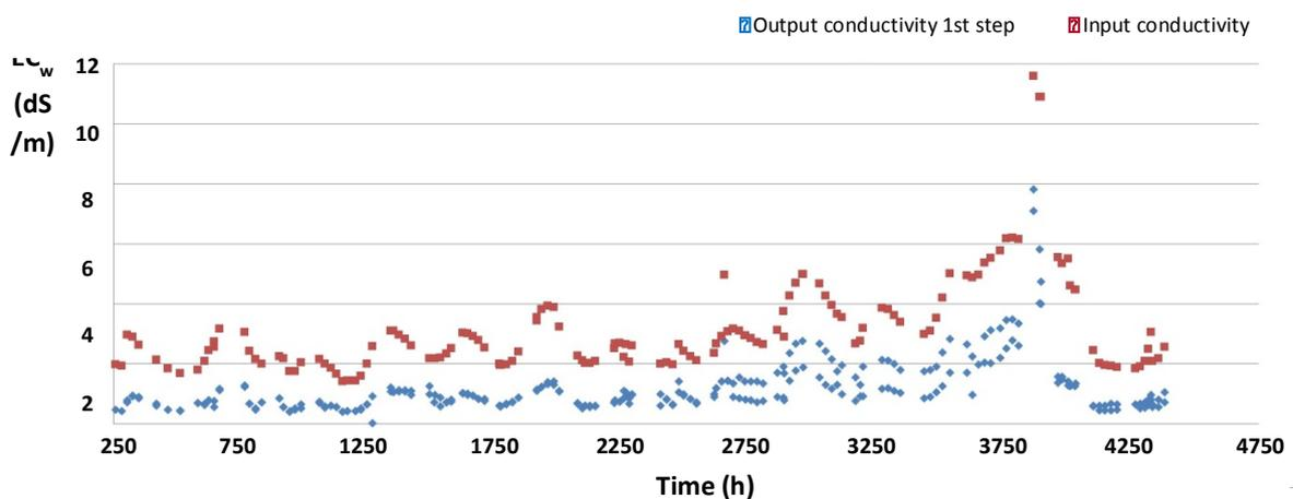
**Figure 1.** Water conductivity reduction by function of fluctuation of inlet salinity with electro dialysis reversal (EDR).
