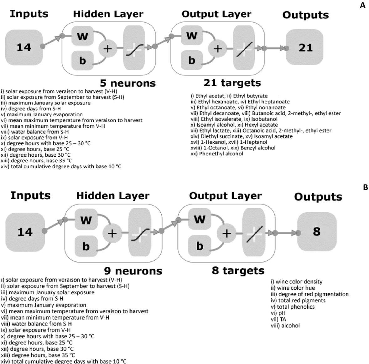
**Figure 1.** Model diagrams showing a the two-layer feedforward networks with sigmoid functions using 14 weather-related parameters and A) 5 hidden neurons and 21 outputs / targets for Model 1, and B) 9 neurons and 8 outputs / targets for Model 2.
