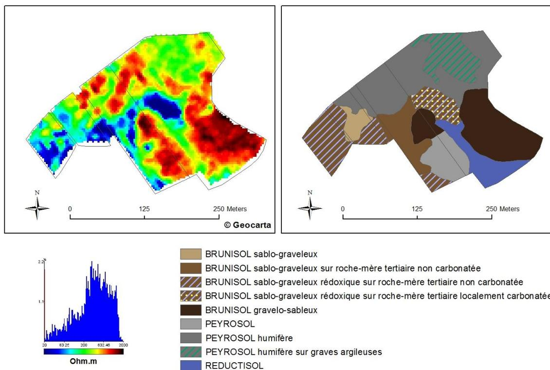
**Figure 1: Example of the use of soil electric tomography (left panel, Geocarta, 75002, France) in the production of soil maps (right panel, van Leeuwen, Roby, Marguerit and de Rességuier, unpublished)**
