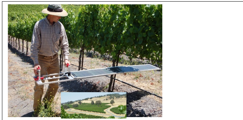
Figure 2: Measurement of light interception by vine canopy in A) a commercial production vineyard in the California Central Coast (courtesy of M. Battany, UC CE Sn Luis Obispo County, CA), and B) one study vineyard in El Dorado County.
