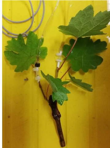
Figure 3: Image of the connection between both shoots and the XYL'EM system.
