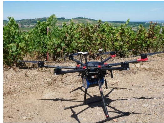
Figure 3: Gamma-ray spectrometer used under a drone in the St Amour vineyard (©CVA 2020).
