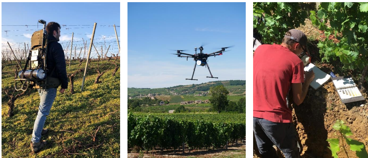
Figure 4: The method combines gamma-ray spectrometer collection and field calibrations (©CVA 2020).
