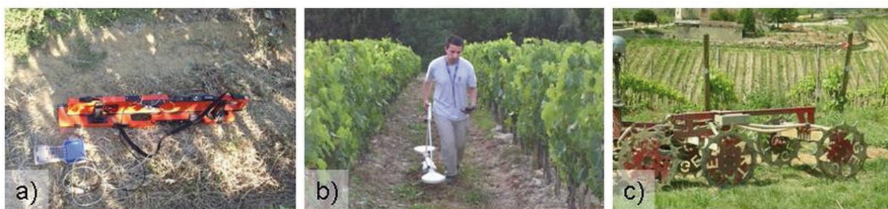
Figure 1: The three proximal sensors used for this work. a) Geonics EM38-DD, b) GSSI Profiler EMP-400, c) Geocarta ARP©.
