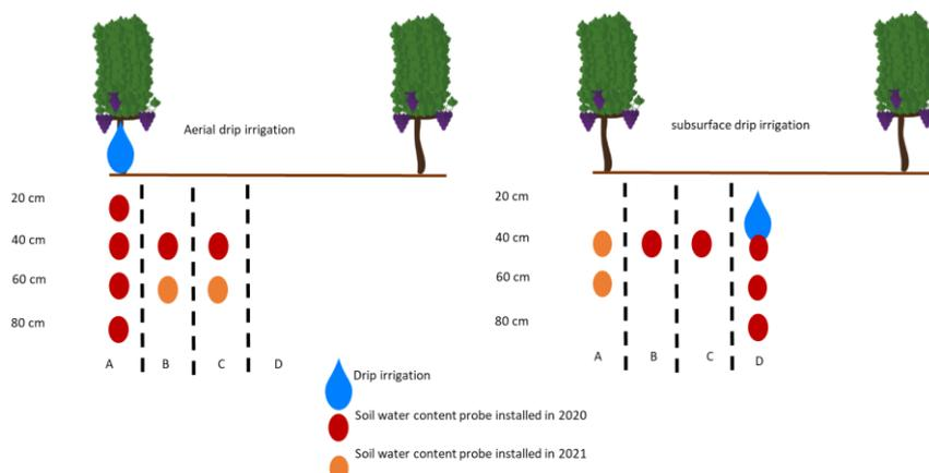
**Figure 1.** Capacitive probes positioning on Aerial Irrigation (AI) and Subsurface Irrigation (SI) treatments
