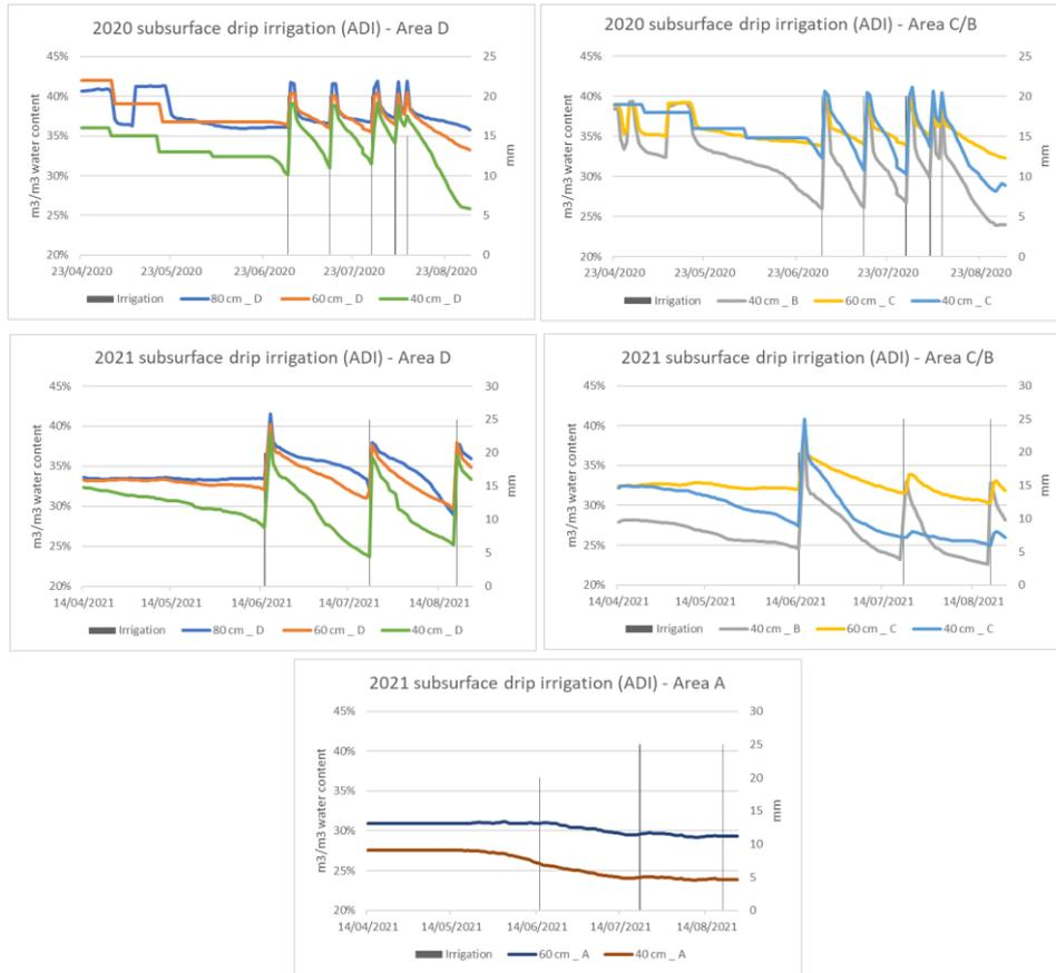
**Figure 3.** Variation of soil moisture on Subsurface Irrigation (SI) at different depth
