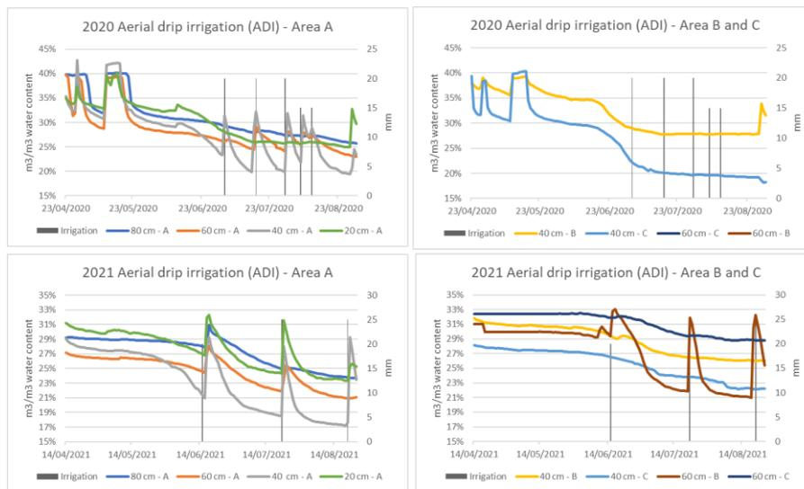
**Figure 2: Variation of soil moisture on Aerial Irrigation (AI) at different depth**
