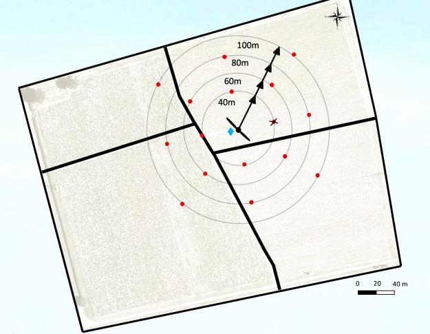
Schematic of the location of the 16 stations (red dots), the 10-m mast (cross), the WM (propeller scheme) and the heater (blue diamond).
