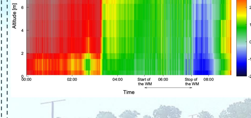
Thermal stratification at the 10 m mast located 40 m away from the wind machine<br/>Night of 2022.02.2500h01h02h03h04h05h06h07h08
