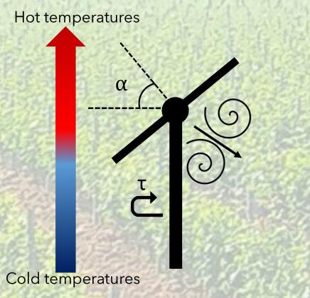
Schematic of the operation of the WM.  $\tau$  is the rotation time and  $\alpha$  is the rotor tilt angle. Adapted from Heusinkveld et al. (2020)
