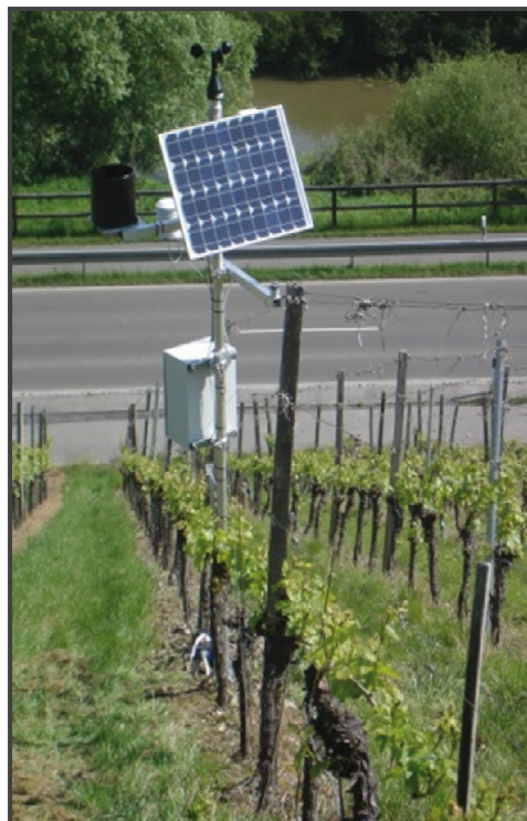
Fig. 2: Meteorological station of Nordheim. The station collects parameters like air and soil temperature, global radiation, precipitation and wind velocity
