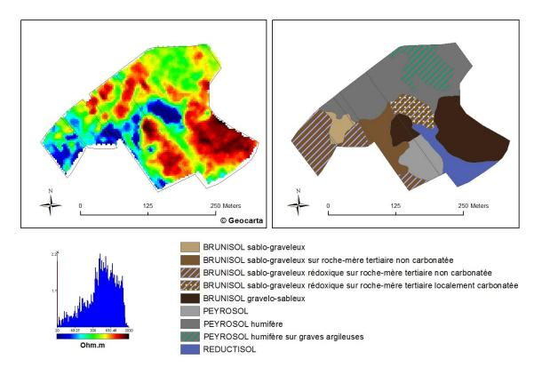
Figure 1: Example of the use of soil electric tomography (left panel, Geocarta, 75002, France) in the production of soil maps (right panel, van Leeuwen, Roby, Marguerit and de Rességuier, unpublished)
