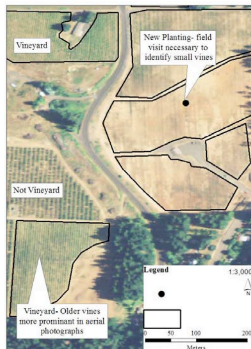
Figure 1: Aerial Photographs from the National Agriculture Imagery Program (NAIP) were used to trace vineyard boundaries once GPS locations were imported into Arc Map.
