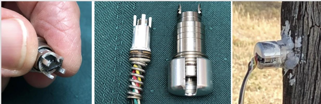
**Figure 1:** The microtensiometer chip (upper left), housed in a protective cylindrical probe exposing the water exchange surface (arrow). Right, the sensor probe and the sleeve that is driven into the stem, provides a drill guide for drilling an installation hole, and an installation in a grape trunk (lower left).
