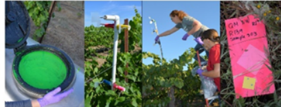
Figure 1. Left - Tracer is added to the sprayer tank for vineyard application. Left Center - Tracer was collected from multiple zones in the canopy. Right Center - Aerial drift deposition was also collected. Right - Drift onto the vineyard floor was collected both for analysis (plastic cards), and for visual comparison (yellow water-sensitive paper).
