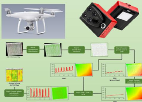
Figure 1. Top: Phantom 4 Pro (left) and Parrot Sequoia multispectral sensor (right). Bottom: new object based imagery analysis (OBIA) process.
