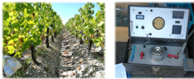
Figure 1. Stem water potential (SWP) and predawn leaf water potential (PLWP) were measured using a pressure chamber
