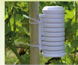
Figure 1 : solar radiation shield housing temperature logger
