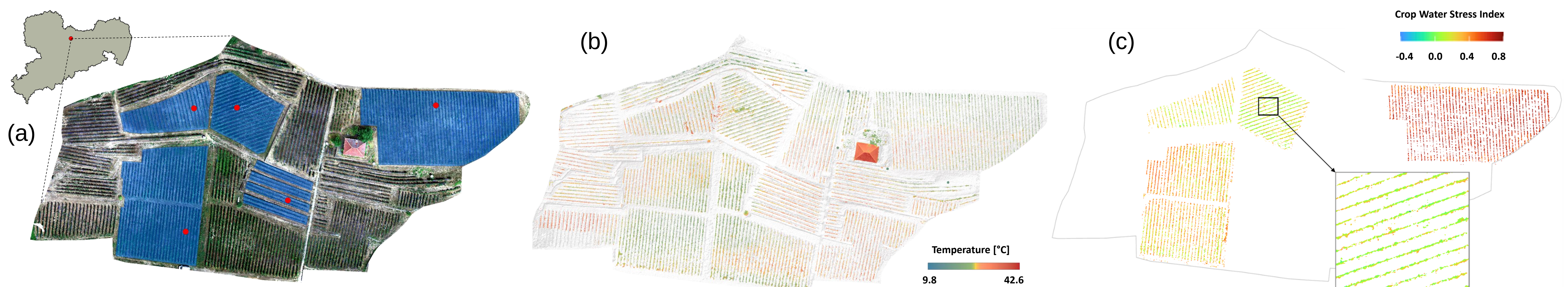
Figure 2: Example data products generated by PyExpress software using automated data pipelines based on the analysis of UAV IR and RGB imagery acquired in a vineyard in Seußlitz, Saxony. (a) Orthophoto of the experimental area. Management zones (blue) and microclimatic stations (red) for further research are shown. (b) Surface temperature map obtained from the example workflow shown in Fig.1. (c) Crop Water Stress Index (CWSI) calculated from grapevine canopy temperature data, filtered using point cloud classification to exclude surrounding soil (Boedeker et al., 2024). Additional outputs generated by PyExpress include point clouds, 3D models, precision maps, and workflow documentation to support advanced agricultural analysis.
